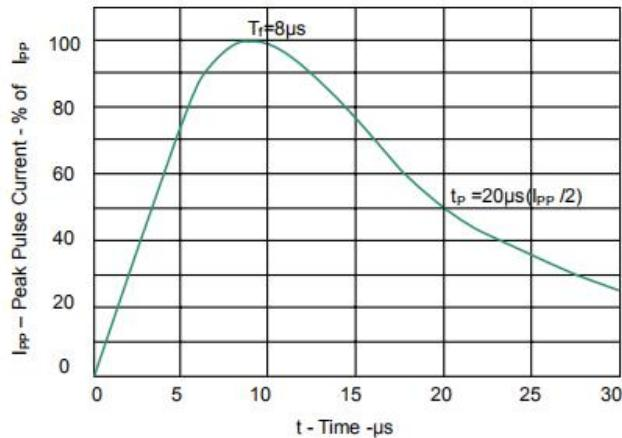
Fig 1.Pulse Waveform
