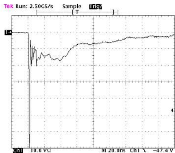
Figure 2. ESD Clamping Voltage Screenshot Negative 8 kV contact per IEC 61000-4-2
